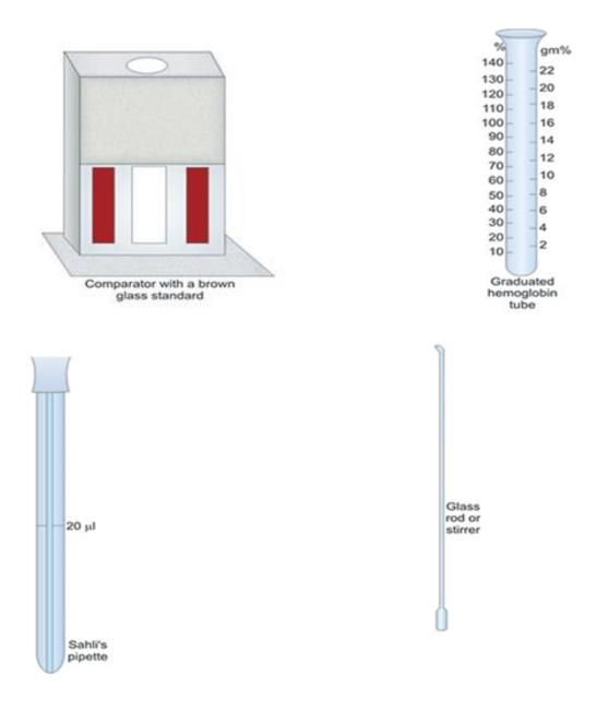
Fig 11: Sahli's Hemoglobinometer
